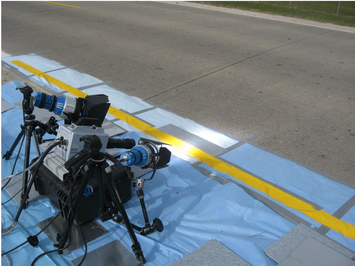
Figure 3.6: High-speed camera setup on side of roadway.
