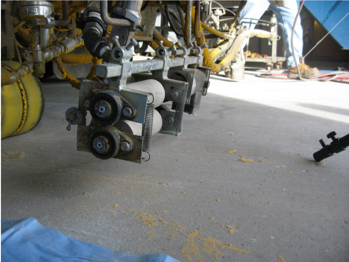
Figure 3.5: Zero-Velocity™ prototype bead dispenser.
