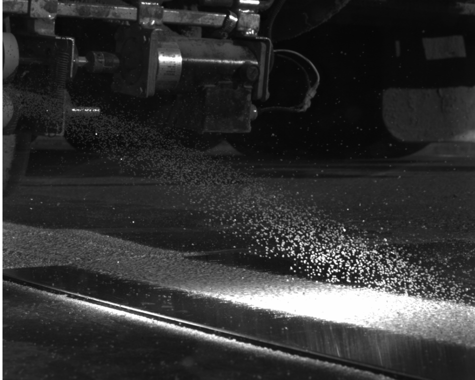
Figure 3.15: Screenshot of Zero-Velocity™ dispersion at 8 mph.
